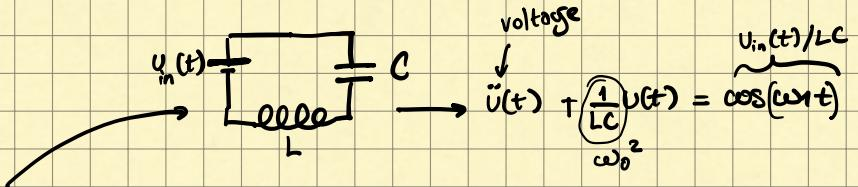
which represents a forced harmonic oscillator or a LC circuit, using Fourier transforms.
